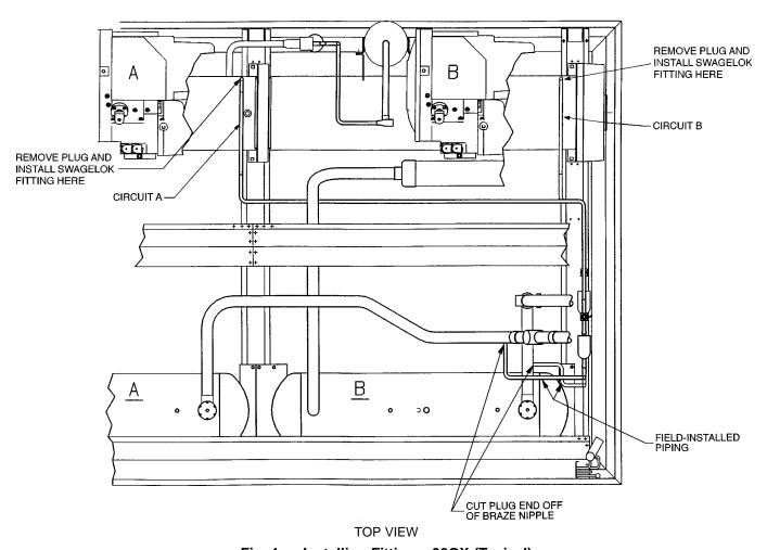
Fig. 1 — Installing Fittings, 30GX (Typical)
